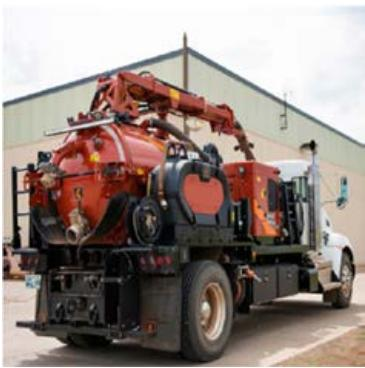
Vacuum Assisted Truck with Pressure Washer
